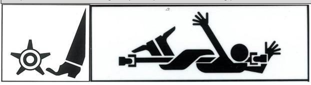
Never use your hands to clear if clogged. Never allow anyone to reach into the rotor housing. The rotor can crush and/or dismember. Keep everyone clear of the rotor until the prime mover engine is off and the hydraulic pressure has been relieved.
